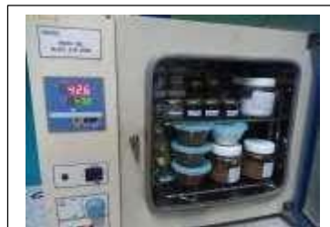
Gambar 31. Uji Cycling test 40°C
